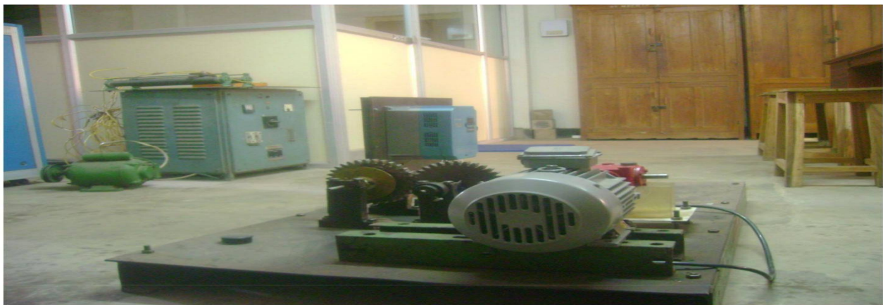
Fig: 11. Motor coupled with the gearbox.
